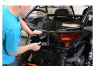
down so the lower holes slide into the spot where the single bolts were removed.
