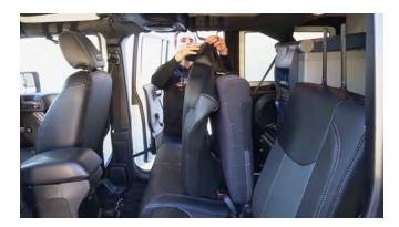
10. Slip the seat cover over the top of the seat, again making sure that the headrest prongs go through the seat cover openings.
