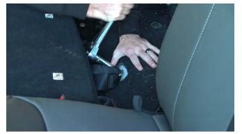
9. Before putting the top cover on, fold the seat down and unbolt the seatbelt.
