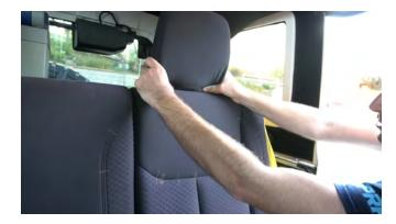
3. Remove the headrests by pushing both release mechanisms near the base of the headrest.
