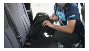
4. Start with the "40" side of the bench and place the bottom cover onto the seat.
