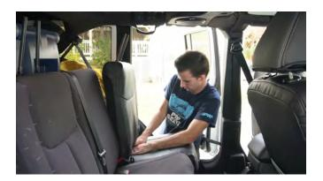
6. Slip the top cover over the seat, making sure to feed the headrest prongs through the openings provided.
