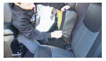
8. For the "60" side of the bench, place the bottom cover over the seat and repeat the same steps as the "40" side.
