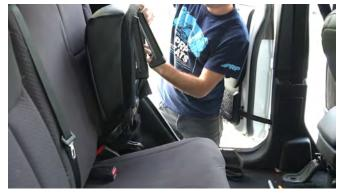
Once the cover is on roughly where you want it to be, begin removing the felt strips on the Velcro and secure them to the carpet material on the stock seat cover.
