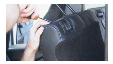
7. Take your finger or the tucking tool provided and push the material under the collapsing handle.
