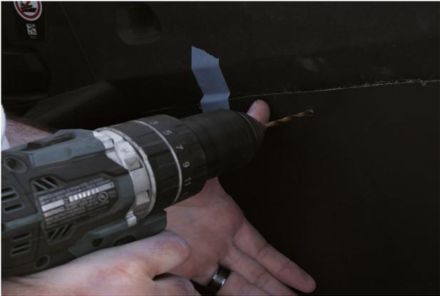
**2. Use a 5/32" drill bit to create holes in the door plastic that the push pins will go into.**
