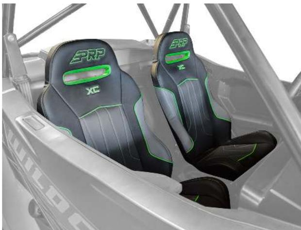
8. **Once the seat is secure to the frame, place it back into the vehicle.**
