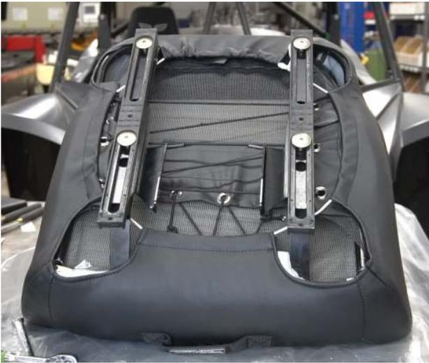
8. Once this is complete, we are going to rebuild the stock slider on the bottom of your PRP Seat.
