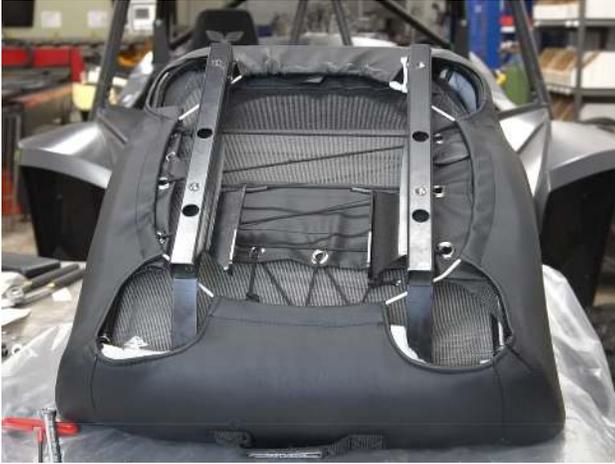
Then place the supplied Square Tube on top of each parallel bar, with the bolt holes lined up. Use the supplied hardware: 4x 3/16" Allen head bolts, 8x washers, and 4x 7/16" nuts to attach each square tube bracket and release handle bracket to the bottom of the seat. Tighten down all 4 bolts/nuts using a 3/16" Allen and 7/16" wrench. [Torque to 144 in-lbs].
