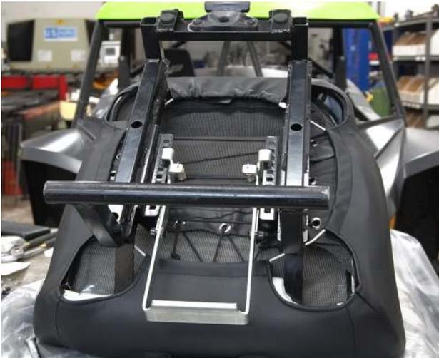
10. Next slide the metal seat base onto the plastic sliders, starting at the rear of the seat, and sliding it forward. The metal base has 4 small holes that should line up with the plastic dots on the sliders. Once the metal base is seated correctly, re-install the 4 stock bolts using a T-25 socket (preferably magnetic tip). [Torque to 36 in-lbs].
