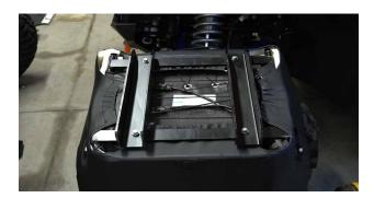
11. The brackets should be oriented with the angled section towards the front of the seat.
