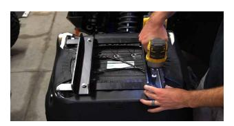
12. Install the brackets to the seat using (4) of the 1/4" bolts, split washer, and flat washers that we supplied. Use a 7/16" wrench or socked to tighten them down.
