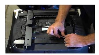
6. Once everything is lined up, install the brackets to the seat using (4) of the 1/4" bolts, split washer, and flat washers that we supplied. Use a 7/16" wrench or socked to tighten them down.
