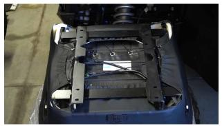
5. Place the Driver Side Brackets onto the bottom of the seat. The smaller bolt holes in the brackets
