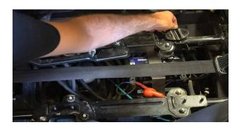
3. Take off both stock brackets, the metal clamps, and the plastic clamps underneath.
