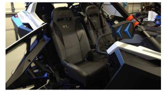
13. Place the PRP Seat into the vehicle. Make sure that both brackets are lined up inside the stock mounts. Make sure the bolt holes on the side of the PRP brackets line up with the bolt holes on the stock mount.
