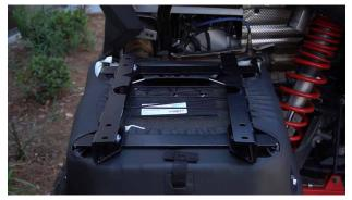
5. Place the Driver Side Brackets onto the bottom of the seat. The smaller bolt holes in the brackets should line up with the bolt holes on
