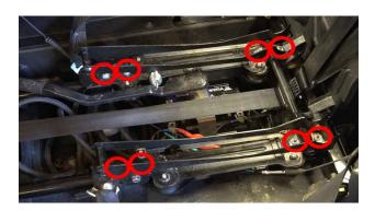
Start by removing the stock seat bracket. Use a 10mm socket to remove the (8) nuts connecting the stock brackets to the sliders.
