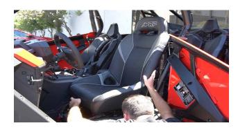
Place the PRP Seat into the vehicle. Make sure that both sliders are lined up even with each other. Make sure all 8 bolts line up with the slots on the bottom of the bracket.
