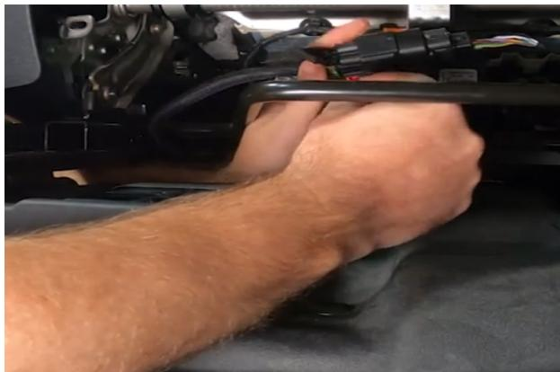
3. There is a wiring connector located under the front of the seat. Using your finger or flat head screwdriver, pop the red clip out of the plastic harness clip and remove it. Then press down on the top of the connector, and pull it apart.
