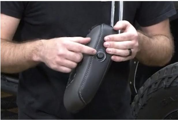
Pull the cover down and over the headrest - use your fingers to depress the foam on the sides to make this easier. Then attach the velcro strips to get it tight. Readjust the cover as needed until the logo is centered.
