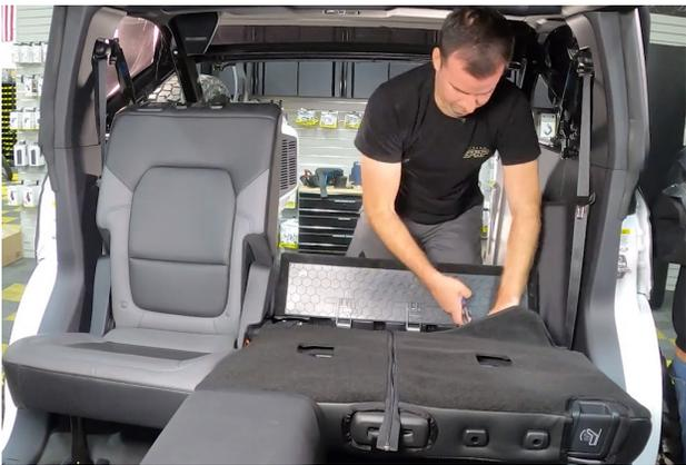
6. On the backside of the seat, lift up the OEM flap. Then pull the PRP cover flap through the center. Pull this flap extra hard, and then attach to the top cover with the velcro strips. You may need to readjust the cover, or tighten the velcro as needed.
