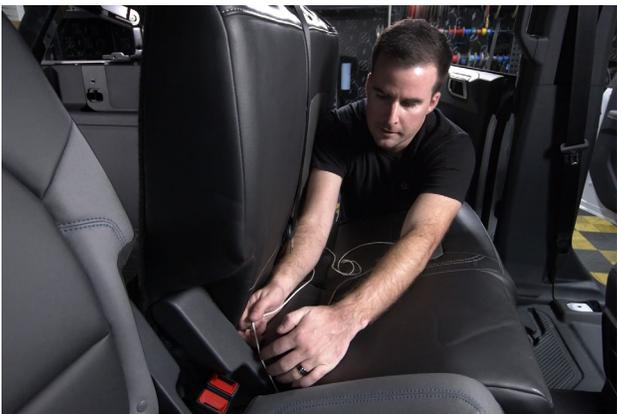
8. Pull down on all the sides and corners of the cover, until its tight all around.
