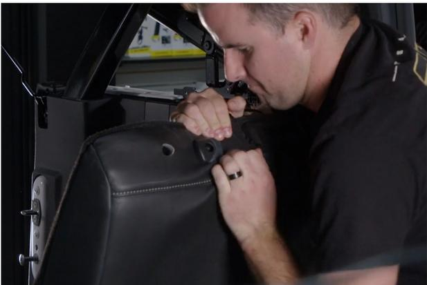
4. On the sides of the seat, push the small flaps behind and around the plastic until they are tight. Then remove the protective fleece, and attach to the back of the PRP cover with the velcro strips.
