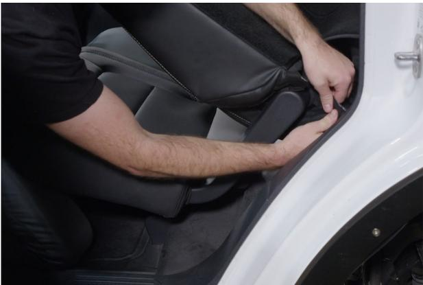
3. Pull the cover down over the seat, and push the flap on the bottom through the center of the seat.
