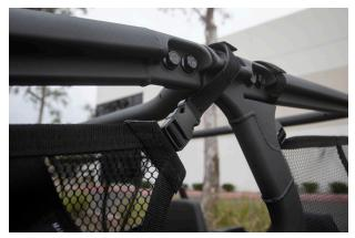
Start by attaching Top-Rear of the net to the cage. Use our supplied Bolt and Nut to attach the strap to the bolt holes on the cage. This strap has a plastic clip included - When you want to get in/out, you can undo this clip and open the door
