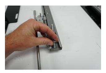
**4.** Attach Hardware to Right Side Slider Grab a pair of sliders and (4x) of the 5/16" Carriage Bolts, Washers, and Nylock Nuts. You will need to use the release handle to open the slider, and slide it backwards to access the square bolt holes on the top side of the slider.
