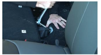
9. Before putting the top cover on, fold the seat down and unbolt the seatbelt using an 18mm socket or wrench.
