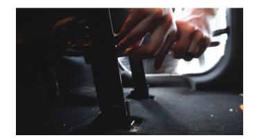
For the rear bench, begin by removing the four bolts holding the bench to the floor using an 18mm socket or wrench.
