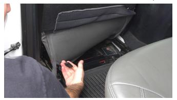
5. Unhook the OEM flap on the back of the seat The top portion of the OEM cover has a flap that wraps around the back & bottom of the seat - Blocking access to the flap you just pushed through.
