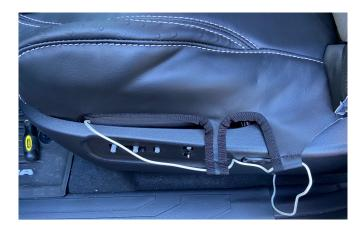
10. Place the cover on and push the back flap through the center of the seat. Wrap the draw strings around the sides of the seat. Tuck the edge of the covers underneath the plastic of the front skirt.
