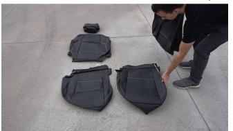
Place the covers out in the sun. This will allow the material to warm up and get rid of most creases formed from being in the box. This also makes it easier to fit the covers over the seat.
