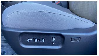
9. Use a flat head screwdriver to pop off all the adjuster buttons. Then remove the two screws hidden behind the buttons. You can then pop the entire side skirt off and forward to remove it.
