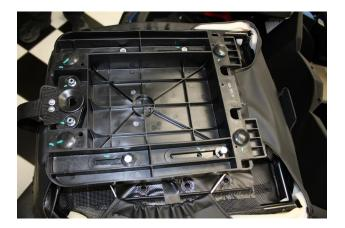
4. Using the 4 – ¼"x20x1" bolts and washers, bolt the plastic pan down to the PRP Seat. The PRP seat has several threaded mounting holes available. Choose witch ever ones line up and get your seat to the desired location. Keep the bolts loose until you test fit the seat back into the vehicle. This way you can get it as far forward as back as you like.
