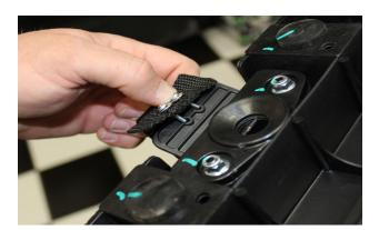
5. In a red plastic bag taped to your seat bag we have included 4 small screws nuts and washers used to attach the webbing at the bottom of the seat to the release latch on your seat pan. Depending on the year of your Z Force you may need to drill the 2 small holes out on your latch so the included screws fit through the holes. This webbing tether is used to release the seat from the vehicle.
