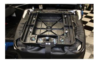
1. Remove the stock seats from the vehicle using the release latch behind the seat.
