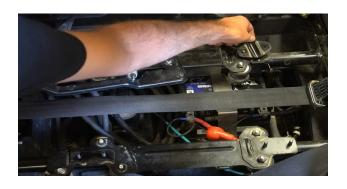
3. Take off both stock brackets, the metal clamps, and the plastic clamps underneath.
