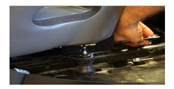
8. Re-Install the (8) stock nuts using a 10mm wrench. Using a wrench with a ratchet-end makes this fast and easy.
