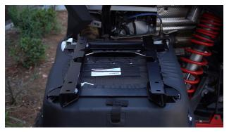
5. Place the Driver Side Brackets onto the bottom of the seat.
