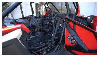
Remove the stock seats from the vehicle. Unlatch the seat and pull it up & out.
