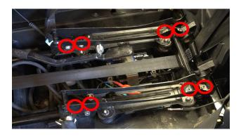
2. Start by removing the stock seat bracket. Use a 10mm socket to remove the (8) nuts connecting the stock brackets to the sliders.
