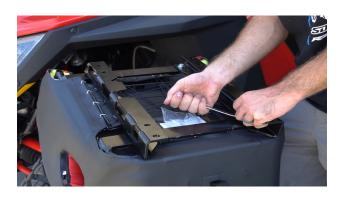
6. Once everything is lined up, install the brackets to the seat using (4) of the 1/4" bolts, split washer, and flat washers that we supplied. Use a 7/16" wrench or socked to tighten them down.
