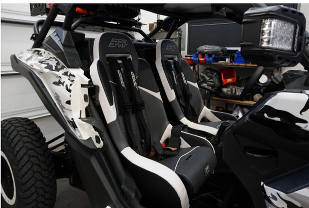
Slide the seat forward to get access to the bolts in the rear. Install any harness lap belts to the two rear bolts, then re-install the OEM nut and tighten down with a 18mm socket.
