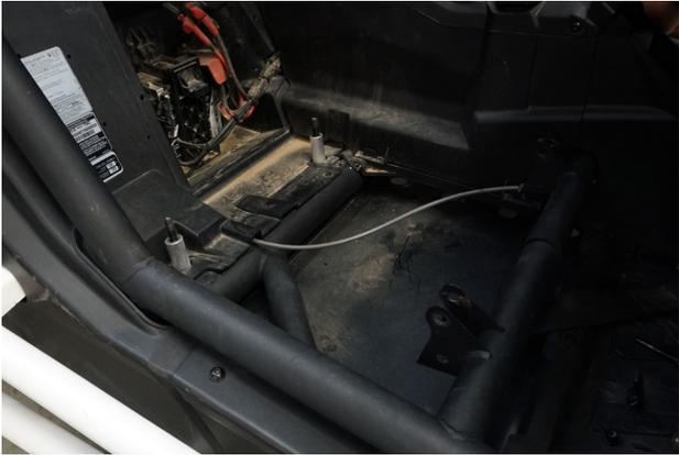
**2. Remove the OEM Slider Rails.**
