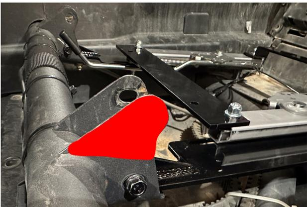
**IMPORTANT** - If you have the mounts in the lowest position, with base mounts also lowered - The front of the seat may hit up against the front OEM mounting brackets when you slide the seat too far forward. To prevent any damage to the seat, you can cut
