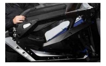
3. Place the bag in-between the metal frame and the plastic panel.
