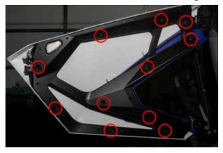
Remove the stock bolts from the door (shown in picture).
