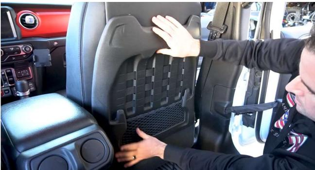
11. For the Rubicon edition -go the back of the seat and pull the cover the rest of the way through. Then take both ends of the cover and attach the velcro strips together. Reattach the plastic Molle back to the seat by pushing it in and up, so that all the clips in the back reattach. Replace the (2) screws using a Phillips Screwdriver.
