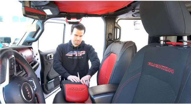
14. Slip the cover over the headrest, making sure that the PRP logo is facing the front. Once pulled all the way down, attach the Velcro strips together to secure the cover to the headrest. Then slip the headrest onto the seat.
