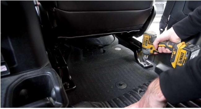
13. Bolt the seat back in with the stock bolts using a T-50 Torx. (make sure to re-attach any wiring harnesses if you removed the entire seat from the vehicle.)
