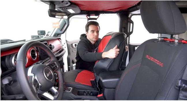
9. Slip the top cover over the seat, making sure the airbag opening faces the outside of the vehicle. Take the bottom flap and feed it through the seat to the back. Around the headrest slots, (and release handle on 2 door models) take the material and push it around and underneath the plastic. Then zip up the side, and tuck the excess zipper underneath the plastic.
