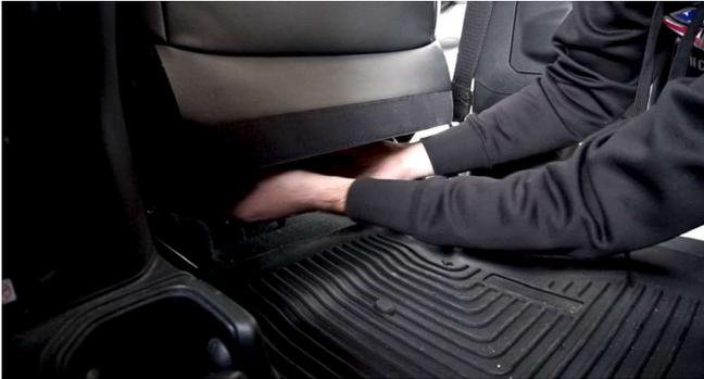
10. For the Sport/Sport S, Sahara, or Moab edition - go the back of the seat and pull the cover the rest of the way through. Lift the stock back flap up, and tuck it underneath the cover. Then take both ends of the cover and attach the velcro strips together. Readjust the covers as needed so that it fits tight, and lines up with the bottom cover.
