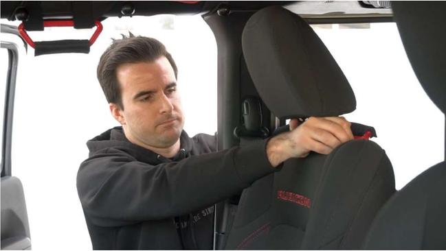
2. Take the headrest off by pushing the two buttons on the seat in and lifting the headrest up and off.
