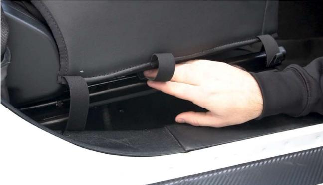
6. Push the elastic bands through the sides of the seat, making sure that they go through on top of the slider (otherwise it will catch). Tip the seat back and do so for the inside bands.
