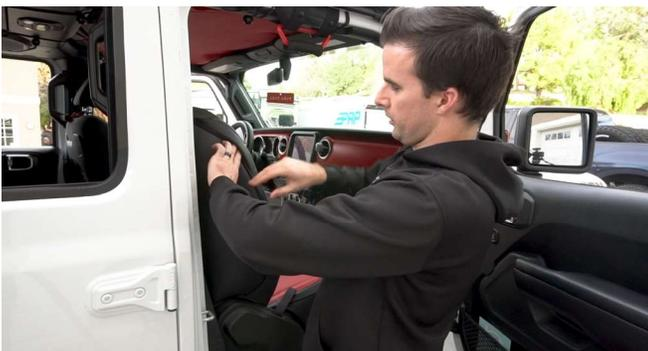
12. On the outside shoulder of each seat is the airbag slot. Take the thinner mesh material and tuck it underneath the cover, so that it lies flat beneath the front side of the seat. Start at the top and work the material in as you go down, so that there are no large wrinkles in the material. **\*\*\*WARNING\*\*\*** if not done properly, the airbag may deploy incorrectly.
