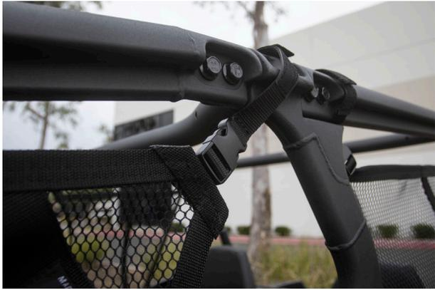
1. Start by attaching Top-Rear of the net to the cage. Use our supplied Bolt and Nut to attach the strap to the bolt holes on the cage. This strap has a plastic clip included - When you want to get in/out, you can undo this clip and open the door
