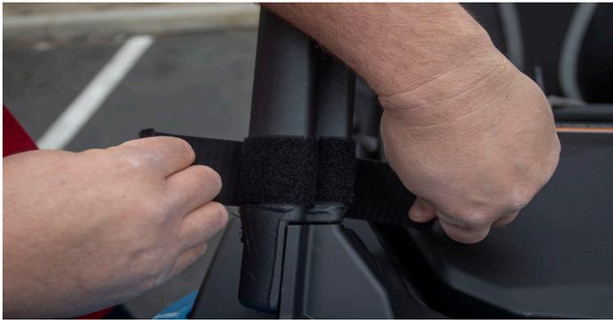
3. Attach the Hook'n Loop strips in the front. These loops have two pieces – an adhesive loop that permanently attaches and stays fixed to the cage, and another cut loop that is attached to the net.
